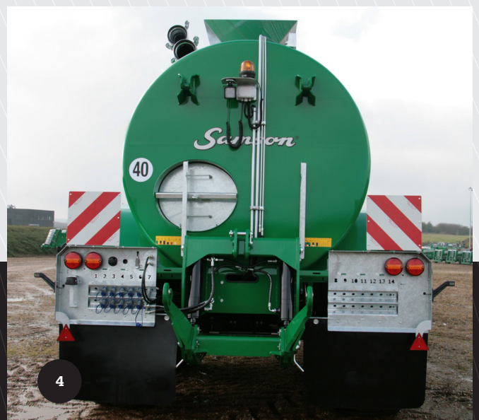
Hydraulic couplings are located where they are easily accessible. The mudguards are optional.
