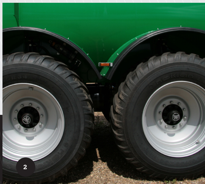
The wheels have a diameter of 165 cm.
